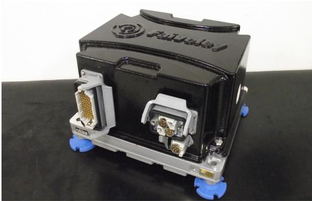
Electronically Controlled Pneumatic (ECP) Brake.
